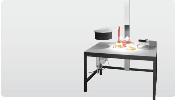
CFR Calibration Facility is designed for the calibration of field pyranometers and albedometers by comparison to a reference instrument of similar type.
