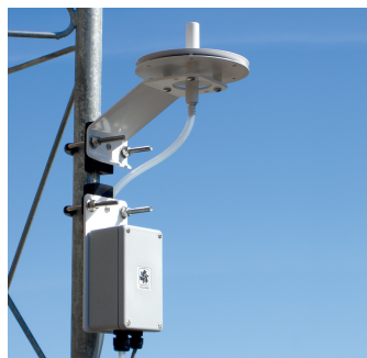
Weatherproof Enclosure and Pressure Port
