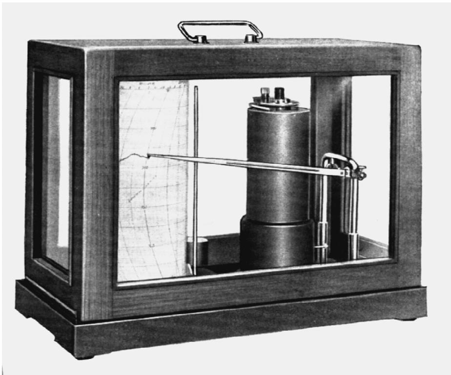
Microbarograph 78m is a highly sensitive measuring instrument for especially sensible and precise recording of atmospheric pressure. Owing to the great height of pen travel of 5mm, for every torr of alteration in pressure, also slightest variations of pressure and fine structures are well to be made out and read with a accuracy of  $\pm 0,1$  torr.
