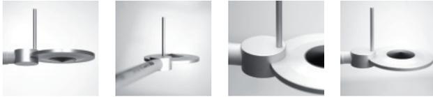
**NR Lite2** is a single-component net radiometer widely used in agriculture and hydrology. The thermopile detector is fitted with a black conical absorber on each side that has a very wide spectral response from the Ultraviolet (UV) to the far infrared (FIR). The black surface is protected by an environmentally resistant anti-stick coating.
