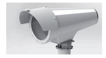
The scintillometer on its own measures changes in refractive index of the atmosphere, Cn<sup>2</sup>, but with the optional meteorological sensor kit it can calculate sensible heat flux. This kit consists of wind speed, temperature and pressure sensors and plugs directly into the X-LAS MkII receiver.
