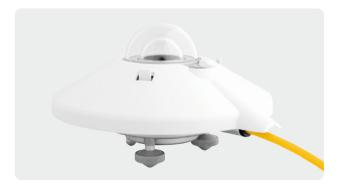
**CMP 11** is an ISO Secondary Standard pyranometer. Compared to the CMP 6 it has better directional response. The detector design is different with faster response and has temperature compensation for greater accuracy with temperature changes. The tilt error and levelling accuracy are also improved.
