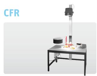
**CFR** Calibration Facility is designed for the calibration of field pyranometers and albedometers by comparison to a reference instrument of similar type.
