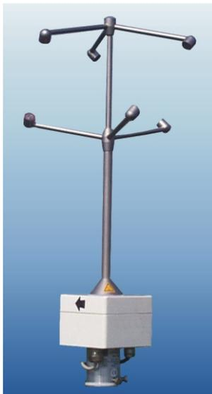
**Ultrasonic Anemometer 3D**
