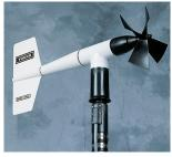
a convenient junction box. The instrument mounts on standard 1 inch pipe. For offshore and marine use, the **Model 05106**, **Wind Monitor-MA** features special waterproof bearing lubricant and a sealed, heavy-duty cable pigtail in place of the standard junction box. Separate signal conditioning for voltage or current outputs is available.
