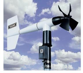
yet lightweight vane with a sufficiently low aspect ratio to assure good fidelity in fluctuating wind conditions. Vane angle is sensed by a precision potentiometer housed in a sealed chamber. With a known excitation voltage applied to the potentiometer, the output voltage is directly proportional to vane angle. A mounting orientation ring assures correct realignment of the wind direction reference when the instrument is removed for maintenance.
