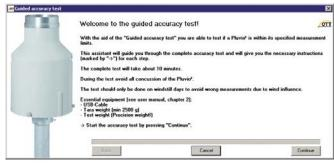
The OTT Pluvio² operating software is menu-driven and allows simple functional checks and accuracy tests on location using a notebook computer. The power supply is simply provided via USB.
