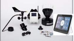
6252 Wireless Vantage Pro2. Includes built-in bubble level for accurate installation. The NEW tipping spoon in our rain collector is self-emptying, corrosion-resistant, and precisely-calibrated for exceptional accuracy.
