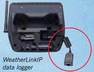
WeatherLinkIP data logger installed in a Vantage Vue console.
