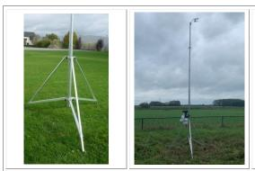
Mast tripods are suitable for portable applications because of their ability to quickly achieve temporary installation. The tripods can be folded in a single movement without the need for tools. Folded, their dimensions are very compact; the diameter of
