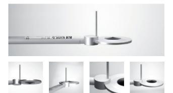
**NR Lite2** is a single-component net radiometer widely used in agriculture and hydrology. The thermopile detector is fitted with a black conical absorber on each side that has a very wide spectral response from the Ultraviolet (UV) to the far infrared (FIR). The black surface is protected by an environmentally resistant anti-stick coating.
