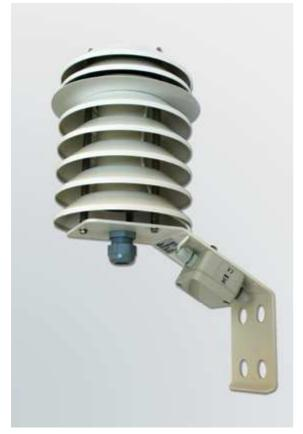
for the protection of an electronic thermometer and / or hygrometer against the influences of weather and radiation. The shield consists of white painted Aluminium. This design ensures a high reflectance and low thermal capacity and thus a very small influence of direct and indirect radiation on the measurement.
