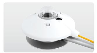
**CMA 6** is an ISO First Class albedometer that uses two CMP 6 pyranometer detector assemblies built into a single housing. An integrated glare screen prevents direct illumination of the lower domes at sunrise and sunset, and a screw-in drying cartridge keeps the interior free from humidity. A mounting rod is fitted to provide easy attachment to a mast in combination with the CMB 1 mounting bracket.
