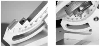
In solar energy applications it is often desirable to measure the 'tilted' global solar radiation at the angle of non-tracking (fixed) photovoltaic panels, in addition to the usual horizontal global radiation measurement. This can be achieved by mounting a pyranometer at the same angle as the fixed PV panel, so that it sees the same incoming solar radiation.
