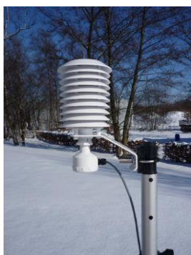
HygroClip 2 - Meteo inserted into a meteorological screen Model 41003
