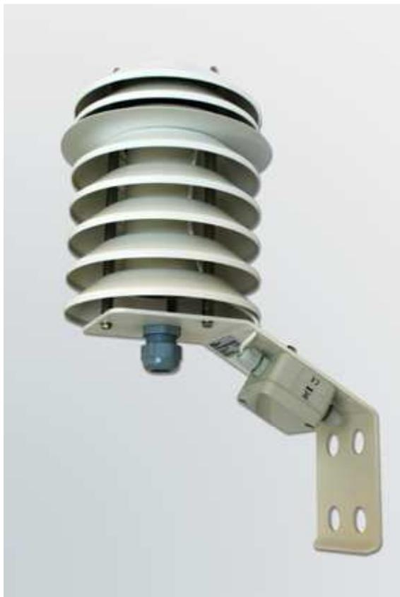
for the protection of an electronic thermometer and / or hygrometer against the influences of weather and radiation. The shield consists of white painted Aluminium. This design ensures a high reflectance and low thermal capacity and thus a very small influence of direct and indirect radiation on the measurement.
