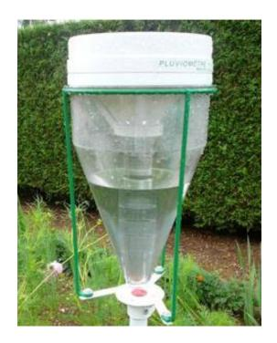
In order to increase the accuracy, especially for the light rain, the system is completed with a central test piece that measures rains up to 8 mm with an accuracy of 0,1 mm.
