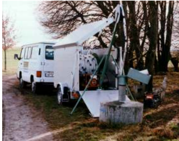
sampling system with 2"-pump up to 250 m depth
