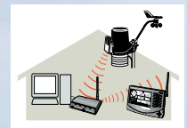
Retransmit from Weather Envoy to console
